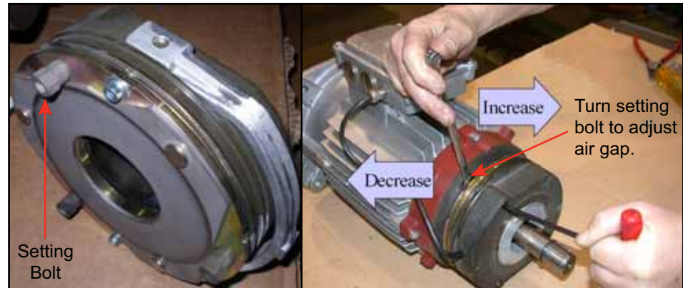
Figure 6-13: Adjusting the Setting Bolt
