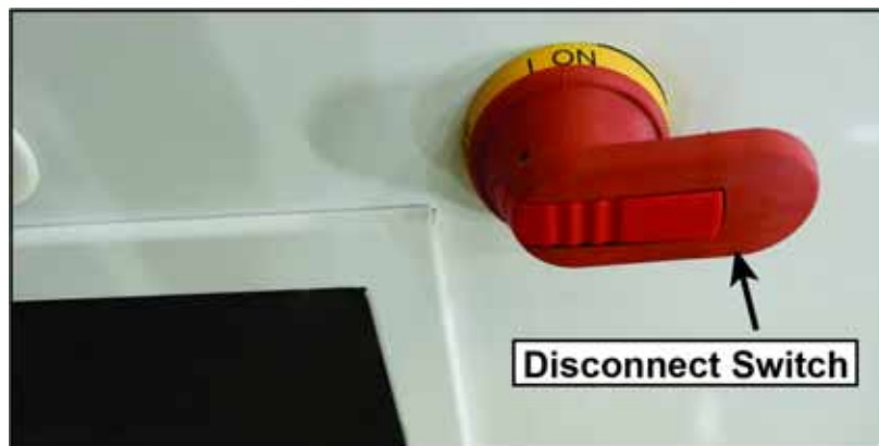
Figure SAFETY-2: Disconnect Switch
