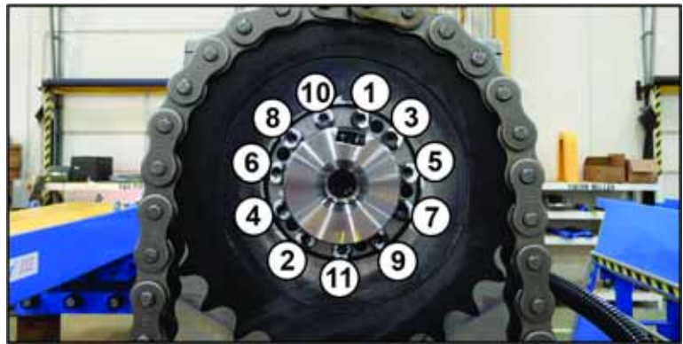
Figure 6-3: Bolt Removal Pattern
